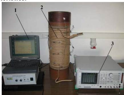
Fig.1 Standard winding and measuring equipment 1. IFRA measuring system; 2. Standard winding; 3. SFRA Network Analyser
