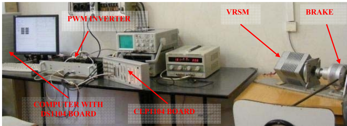
Figure 6: Picture of the proposed experimental test bench
