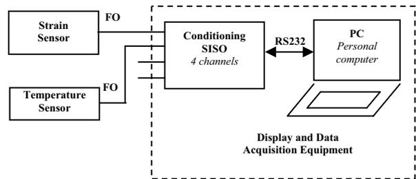
Fig.6. – Fiber Optic Industrial Force/Mass measurement with temperature compensation.
