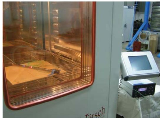
Fig.11 – Temperature variation test in climatic chamber Vötsch.
