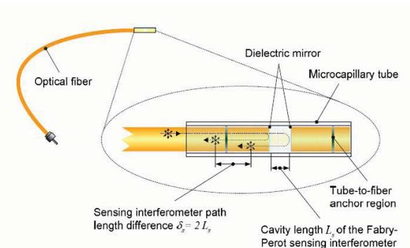
Fig. 2. – Principle of strain sensor integrated in fiber optic
