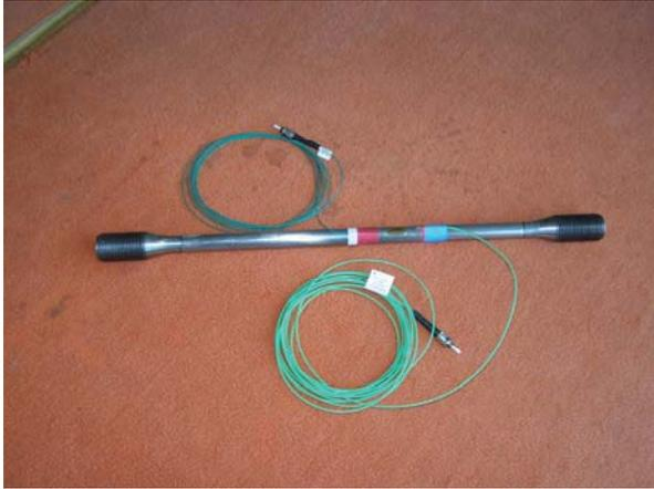
Fig. 7 – 100 kN force transducer with FO sensor (tension).
