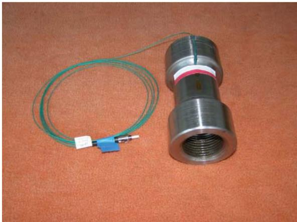
Fig. 8 –200 kN force transducer with FO sensor (tension/compression).
