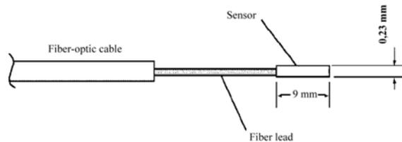
Fig. 1. – Strain sensor type OSP-A.
