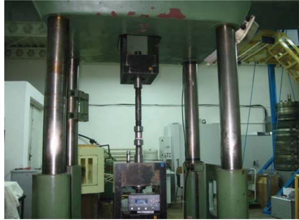
Fig. 9 – Test setup for the de 200 kN transducer in the 1000 kN machine
