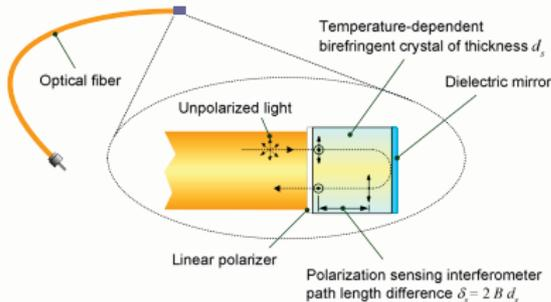
Fig. 4. – Principle of interferometric temperature sensor integrated in fiber optic
