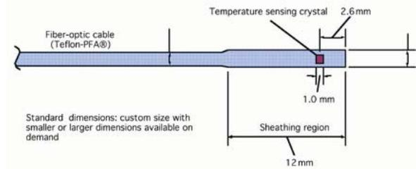
Fig. 3. – Temperature sensor type OTP-A.
