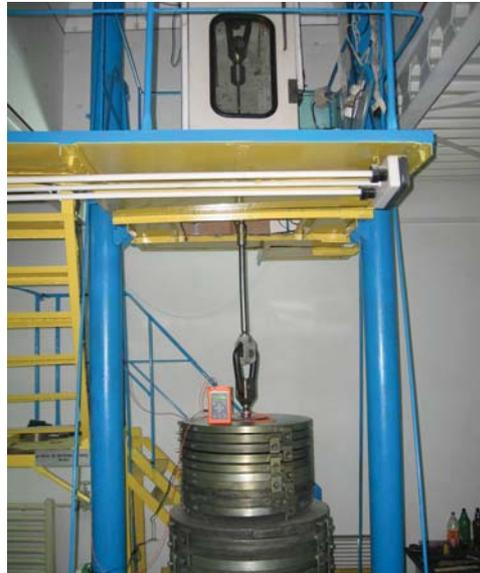
Fig. 10 – Test setup for the de 100 kN transducer in the 1000 kg machine
