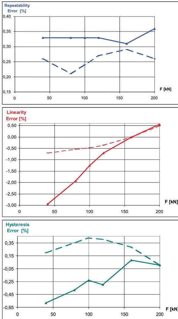
Fig.13-Measurement errors of the 200 kN transducer (T/C) (solid line - compression, dotted line - tension)
