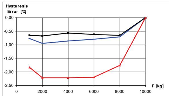
Fig.12 - Measurement errors of the 100 kN transducer (T) (blue - 0°C  $\pm$  1°C, black - 21°C  $\pm$  1°C, red - 50°C  $\pm$  1°C)
