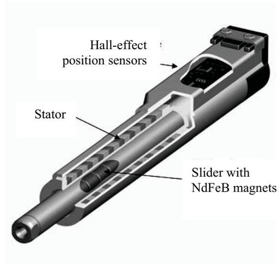
Figure 1: Two-phase TLBLPMA prototype under study (provided by LinMot, Inc.)
