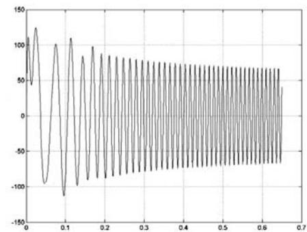
Figure 7: The current  $i_A$  of the first phase.
