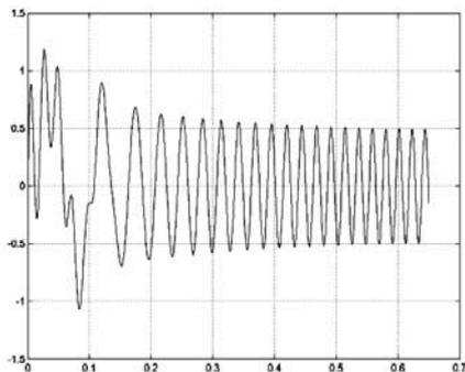
Figure 3: The stator flux in mobile d-q coordinate system
