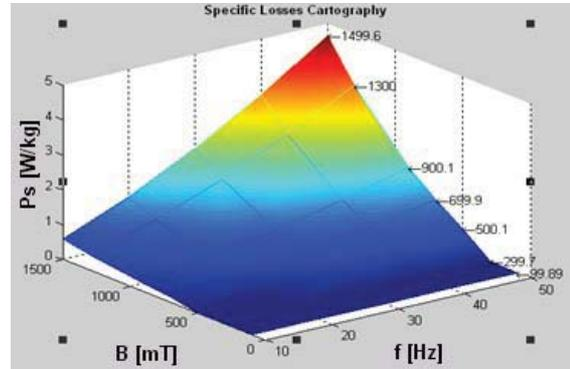
Figure 2: 3D magnetic losses cartography for ER-L sample.
