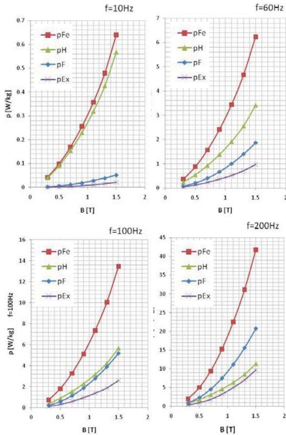
Figure 4: Raised curves of separated magnetic losses for ER-T sample.
