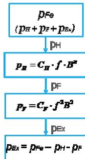
Fig. 5: Logic diagram of specific losses calculation.
