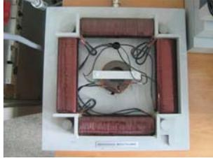
Figure 1: Epstein frame measurement system.
