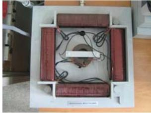
Figure 1: Epstein frame measurement system.
