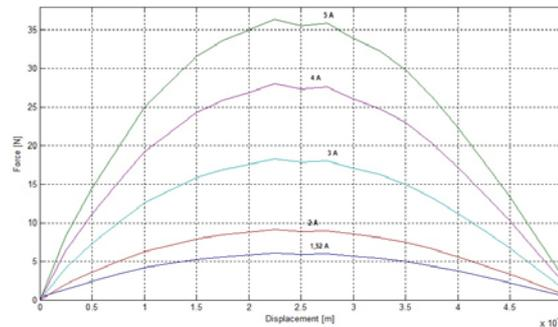
Figure 13: Force profile for proposed tubular motor at various energizing phase currents and positions
