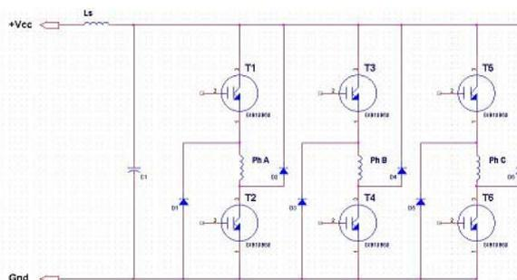
Figure 8: Two Quadrant synchronous chopping converter topology
