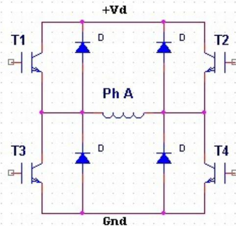
Figure 6: One phase of full H-Bridge converter
