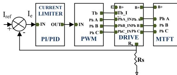
Figure 12: Block diagram of PWM current regulator
