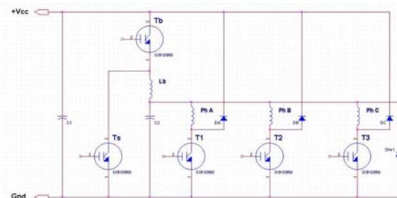
Figure 7: Converter topology with a synchronous buck converter on the front end
