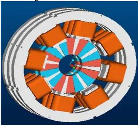
Figure 3: One 3- phase module of MTFTM with active mover
