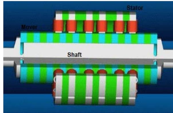
Figure 4: 90 Deg section from MTFTM
