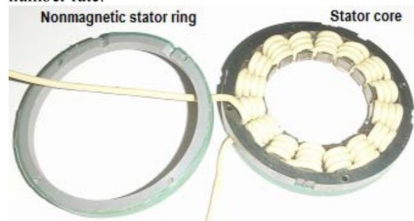
Figure 1: Nonmagnetic stator ring and stator core with coil
