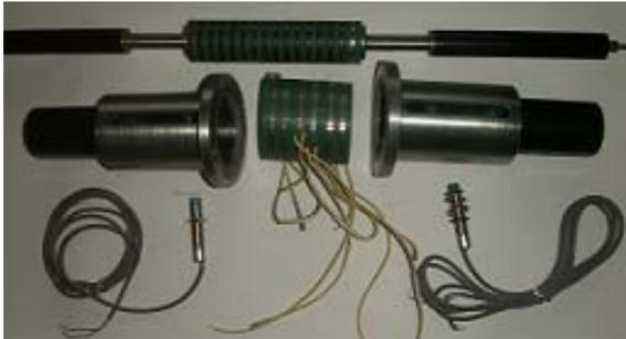
Figure 5: Two modules 3- phase MTFTM disassembled
