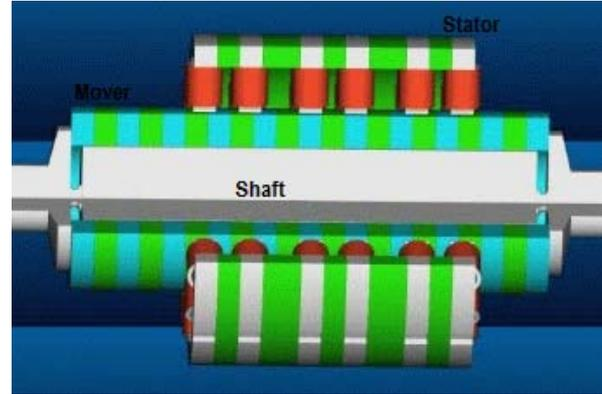
Figure 4: 90 Deg section from MTFTM
