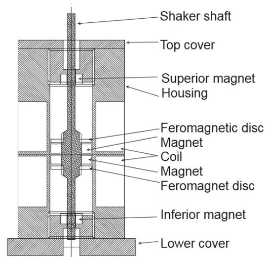
Figure 5: Principle of vibration generator scheme.
