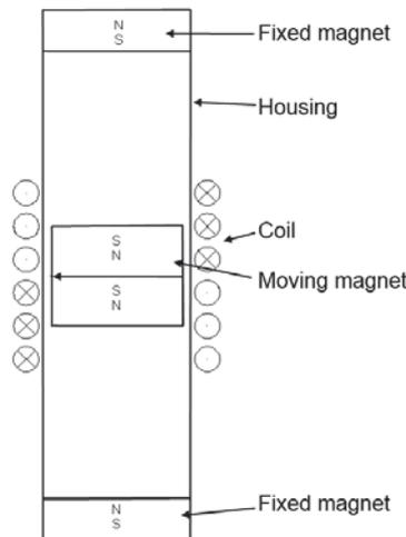
Figure 6: Principle of harvesting generator scheme.
