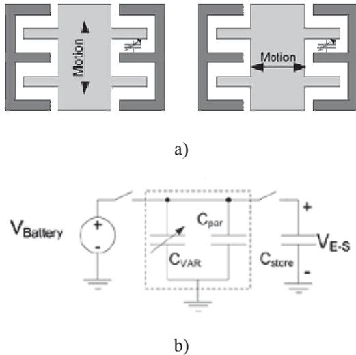
Figure 1: a) Principle of electrostatic conversion scheme, b) electrostatic conversion equivalent circuit.
