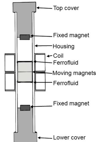
Figure 7: View in section for experimental model of harvesting generator.
