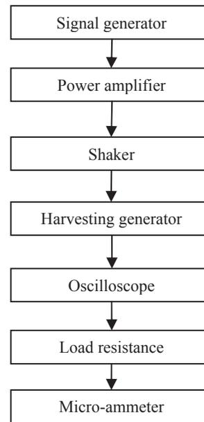
Figure 4: Principle scheme of the harvesting energy system from vibration.
