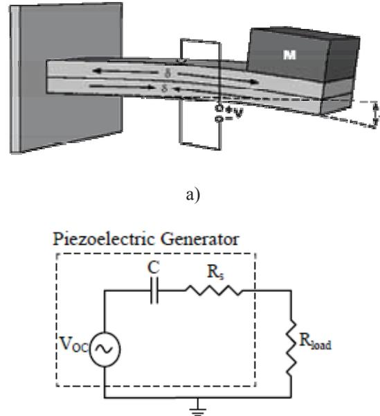
Figure 2: a) Principle of piezoelectric conversion scheme b) piezoelectric conversion equivalent circuit.
