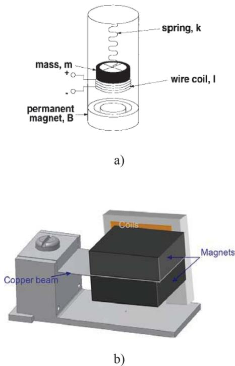
Figure 3: a) Principle of electromagnetic generator scheme with spring; b) Principle of electromagnetic generator scheme with console.
