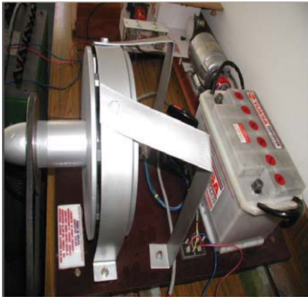
Figure 1: Synchronous machine with axial magnetic field, with double air gap (disk topology) made in the Laboratory of Electromechanical Converters (UDJG)
