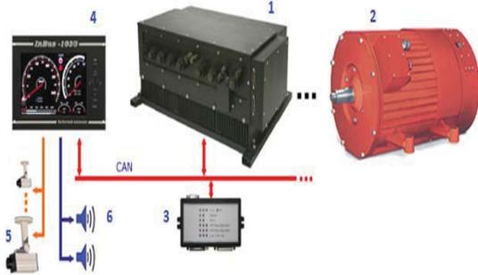
Figure 2. Modular structure of the control system.
