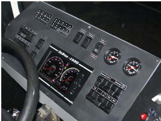
Figure 3. InBus-103G graphic board panel.
