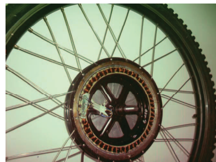
Fig.1. The studied synchronous motor with permanent magnets
