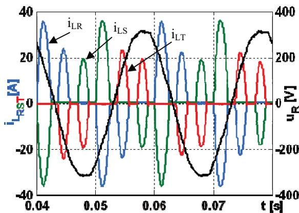
Fig. 11. The grid voltage and the unbalanced non-linear load currents
