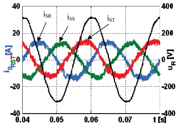
Fig. 13. The grid voltage and the source currents for partial compensation
