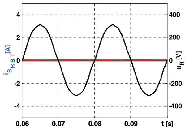
Fig. 3. The grid voltage and the source currents for total compensation
