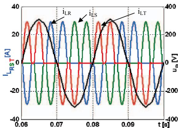
Fig. 2. The grid voltage and the non-linear load currents
