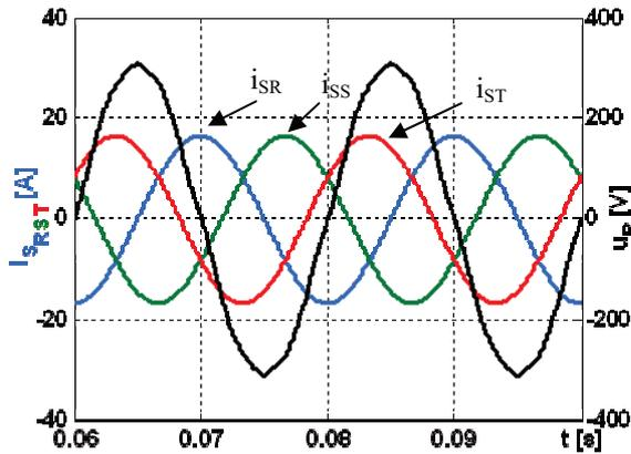
Fig. 4. The grid voltage and the source currents for partial compensation
