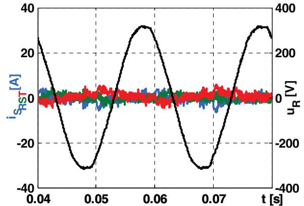
Fig. 12. The grid voltage and the source currents for total compensation
