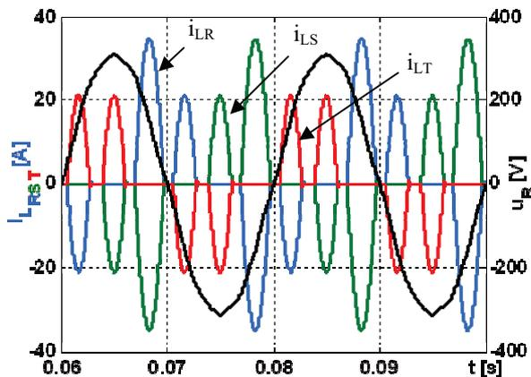
Fig. 5. The grid voltage and the unbalanced non-linear load currents
