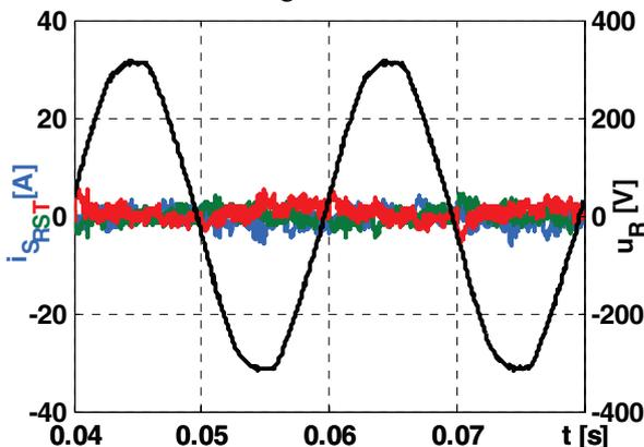
Fig. 9. The grid voltage and the source currents for total compensation
