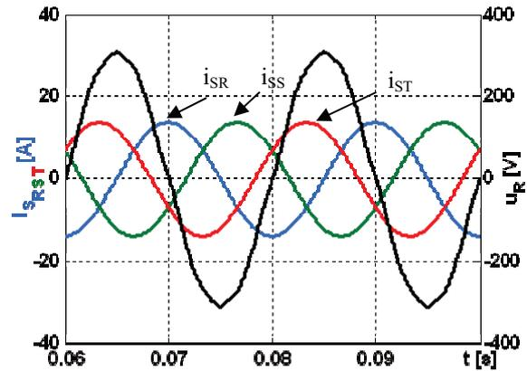
Fig. 6. The grid voltage and the source currents for partial compensation
