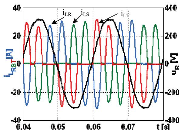
Fig. 7. The grid voltage and the non-linear load currents
