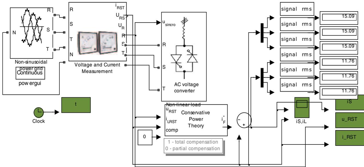
Fig. 1. The virtual filtering system
