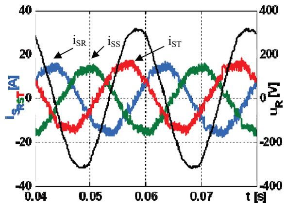
Fig. 10. The grid voltage and the source currents for partial compensation
