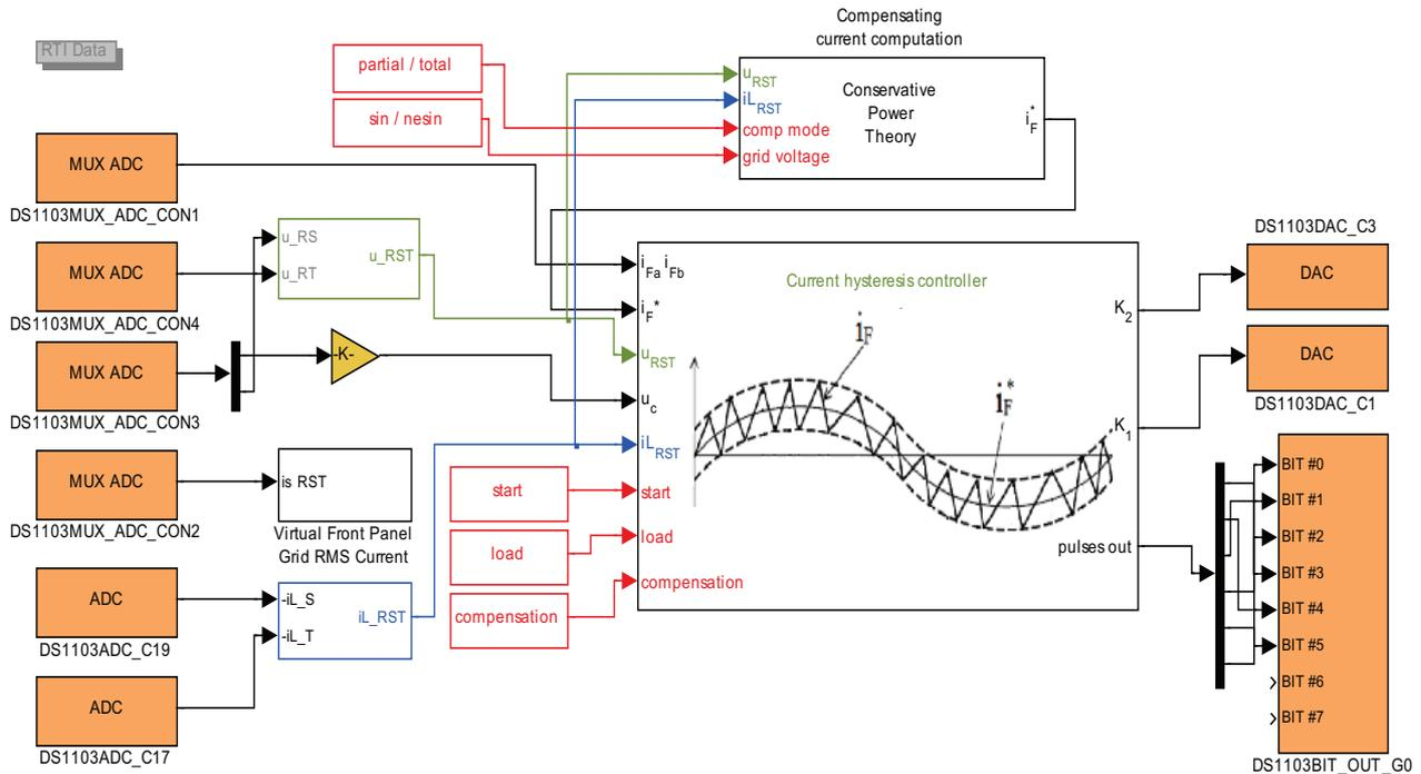
Fig. 8. The Simulink model which implements the active filter current computation and control algorithm
