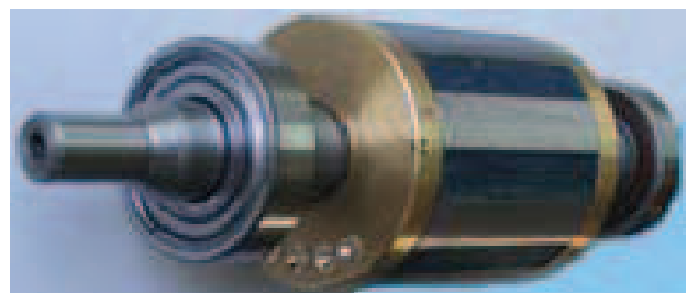
Fig. 21. PMSM with flux concentrator rotor PMSM-FC
