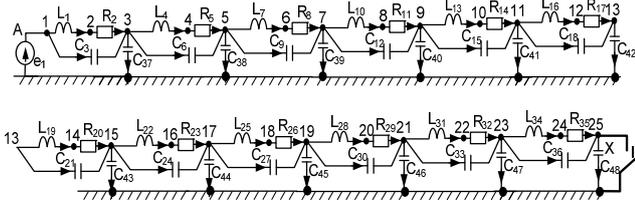
Fig. 3. RLC Ladder Network for over-voltage study when the neutral point either insulated (open breaker) or connected to the ground (closed breaker).
