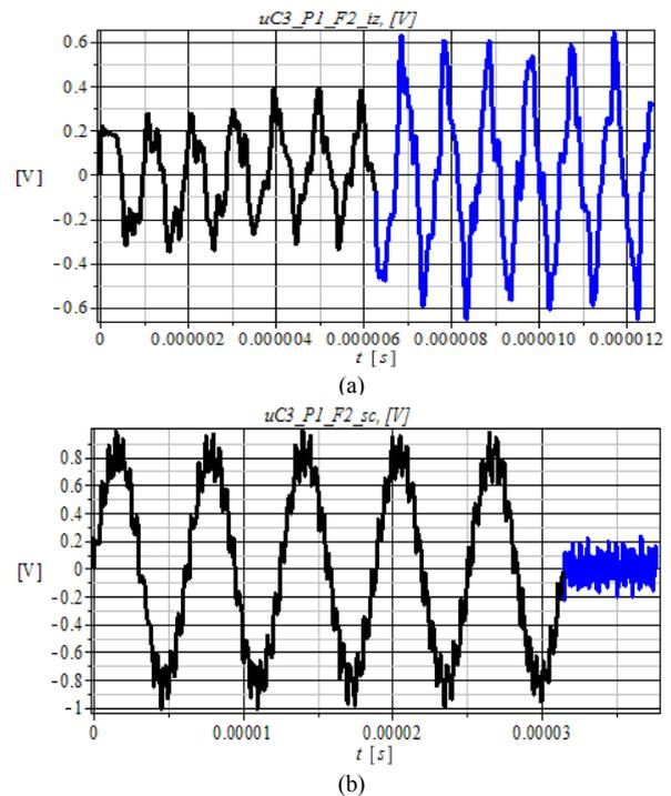
Fig. 4. Time variation of the voltage  $u_{C3}$  for  $\omega_2 = 10^6 \text{ rad/s}$ : a) winding with isolated neutral; b) winding with grounded neutral.
