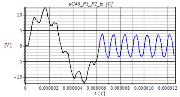
Fig. 6. Time variation of the voltage  $u_{C48}$  for  $\omega_2 = 10^6$  rad/s and winding with isolated neutral
