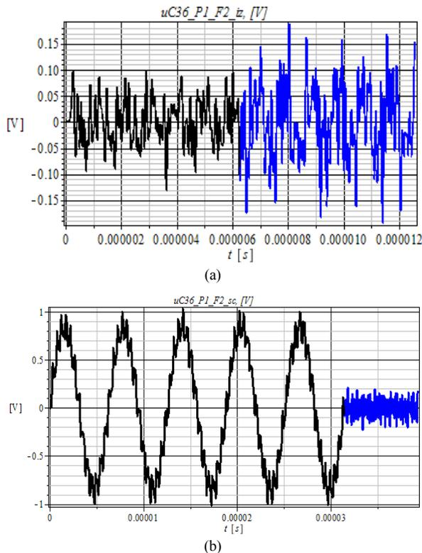
Fig. 5. Time variation of the voltage  $u_{C36}$  for  $\omega_2 = 10^6$  rad/s: a) winding with isolated neutral; b) winding with grounded neutral.
