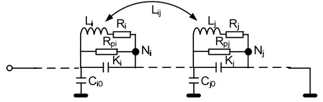
Fig. 2. The Disk Coils i and j from the *RLC* network [2].
