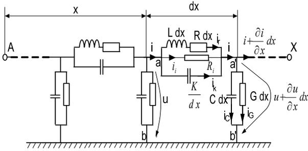
Fig. 1. The equivalent circuit for the model with distributed parameters.
