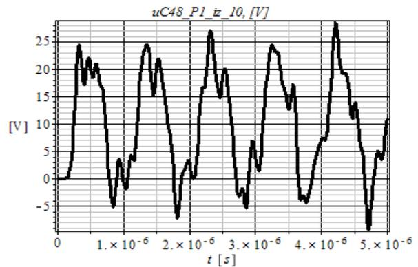
Fig. 10. Time variation of the voltage  $u_{C48}$  for step overvoltage and winding with isolated neutral.
