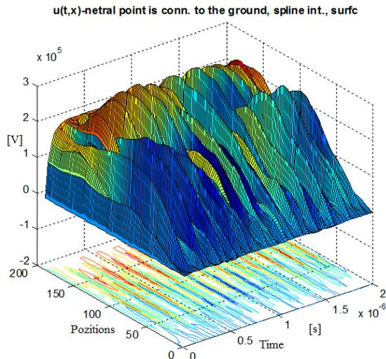
Fig. 12. Time variation of the over-voltage  $u(t,x)$  with isolated neutral.
