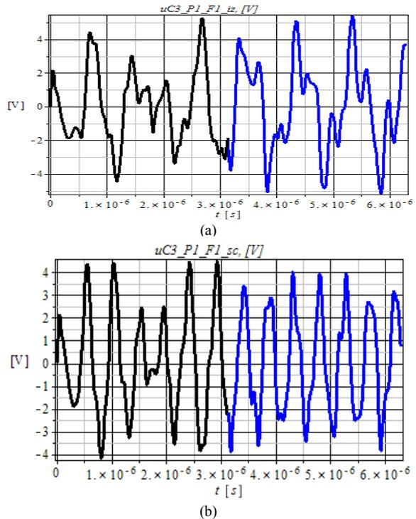
Fig. 7. Time variation of the voltage  $u_{C3}$  for  $\omega_1 = 10^7$  rad/s: a) winding with isolated neutral; b) winding with grounded neutral.
