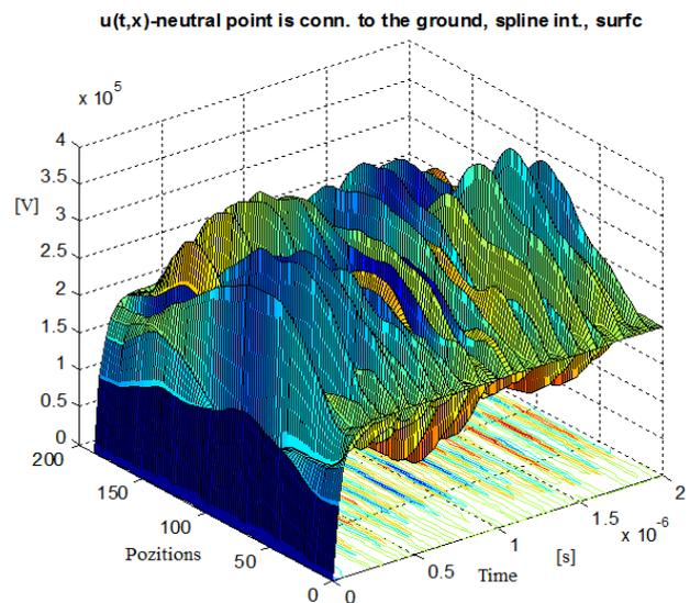
Fig. 11. Time variation of the over-voltage  $u(t,x)$  with grounded neutral.
