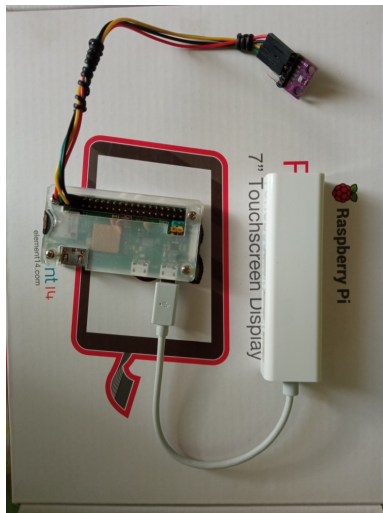
Fig. 8. Sensors, Raspberry Pi Zero and power bank.
