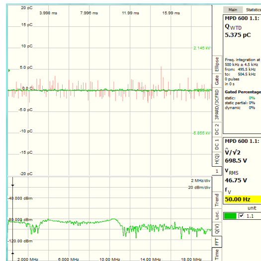
Fig. 7. Frequency spectrum of 5 pC pulse (500 kHz ± 4.5 kHz filter at PD measuring system).
