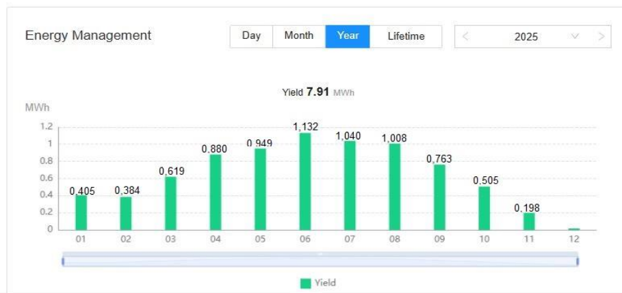
Fig. 15. Monthly energy production from the on-grid PV system measured during the year 2025
