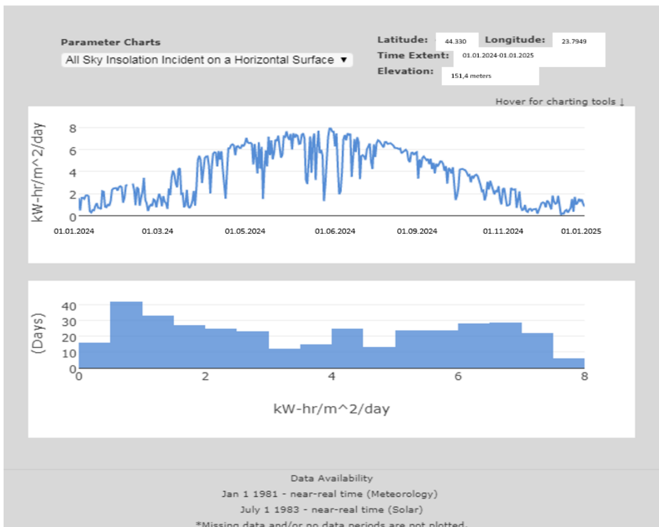
Fig. 5. Annual solar radiation at ground level of approx. 1347 kWh / m 2 .year - 44.3302 ° N (lat) x 23.7949 ° E (long), 01.01.2024-01.01.2025) (NASA Forecast of Worldwide Energy Resource POWER Higher Resolution Daily Time Series 1/2 x 1 / 2 degree, Climatology Resource for SSE-Renewable Energy)
