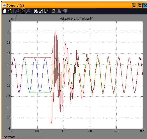
Fig. 10. Voltages at the end of the two lines and the source for other line length [V].
