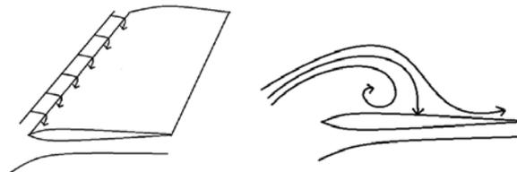
Fig. 1. Appearance and development of vortices on extrados.
