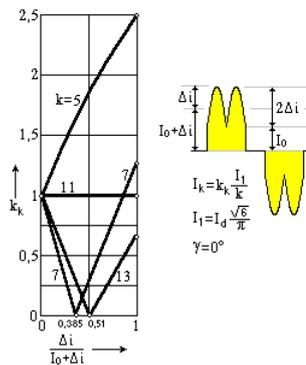
Fig.6. The modify of the harmonics depending on current ripple.
