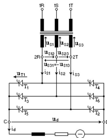
Fig.1. The three-phase bridge rectifier
