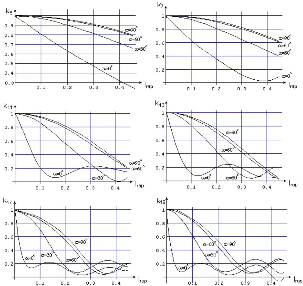
Fig.2. Change of the coefficients  $k_k$  based on  $I_{rap}$ , for different values of the command angle.
