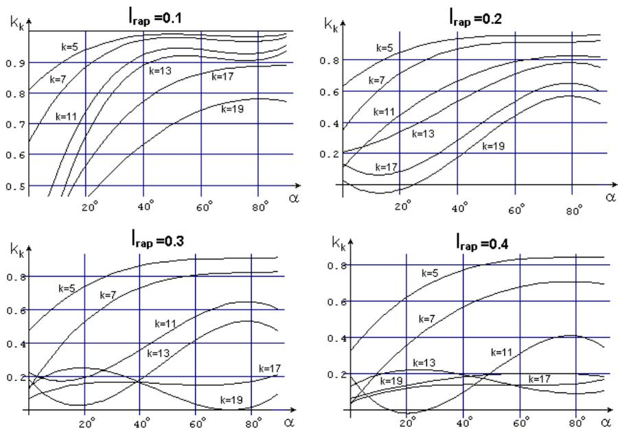
Fig.3. The influence of the command angle on the parameter  $k_k$ .
