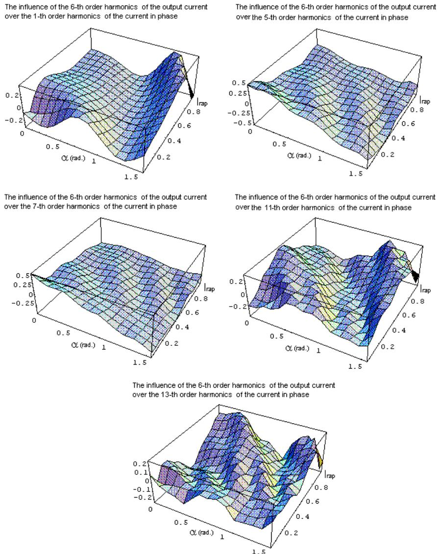
Fig.4. The influence of the harmonics 6 of the current rectified over the current from charging phases.
