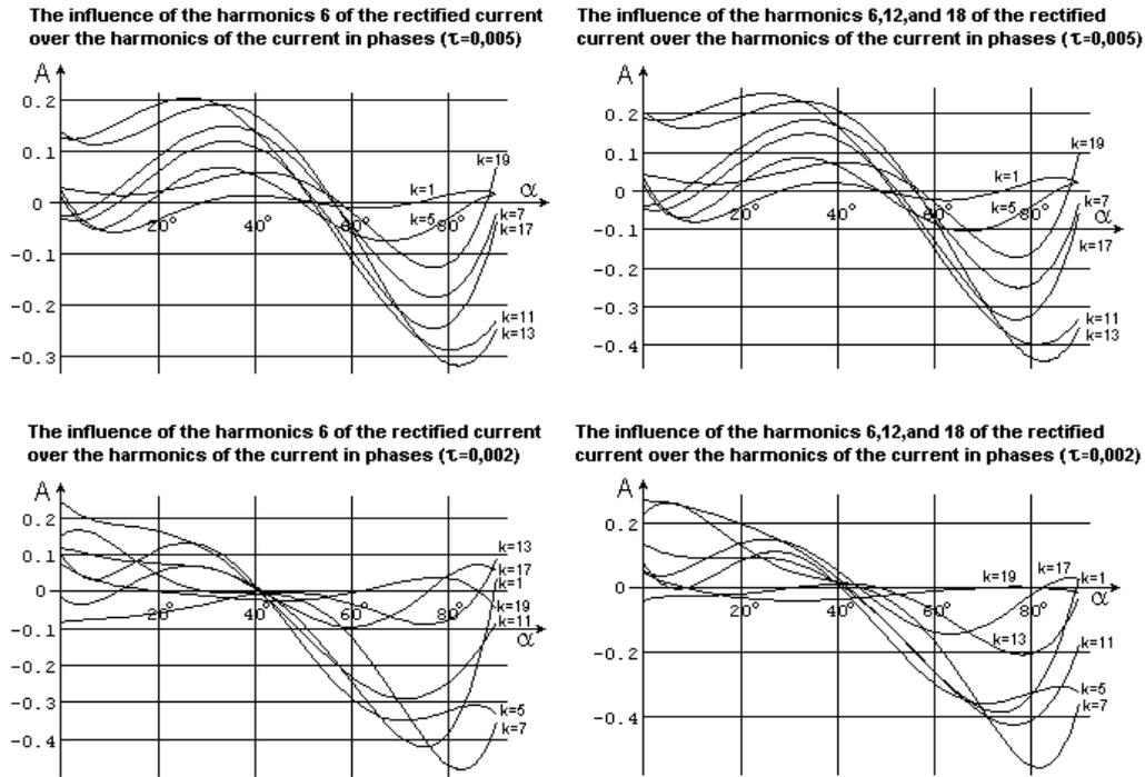
Fig.5. The influence of the harmonics of the rectified current over the harmonics of the current in charging phase.
