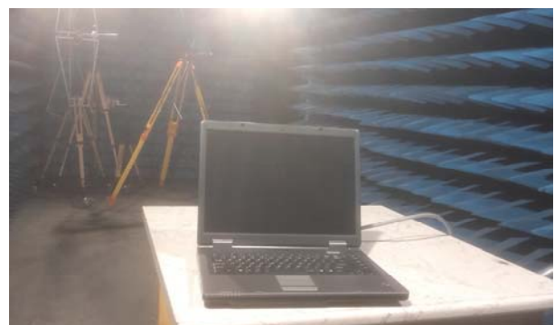
Fig. 6. Placing the equipment in the SAC, in compliance with CISPR 16-4-3 Standard.
