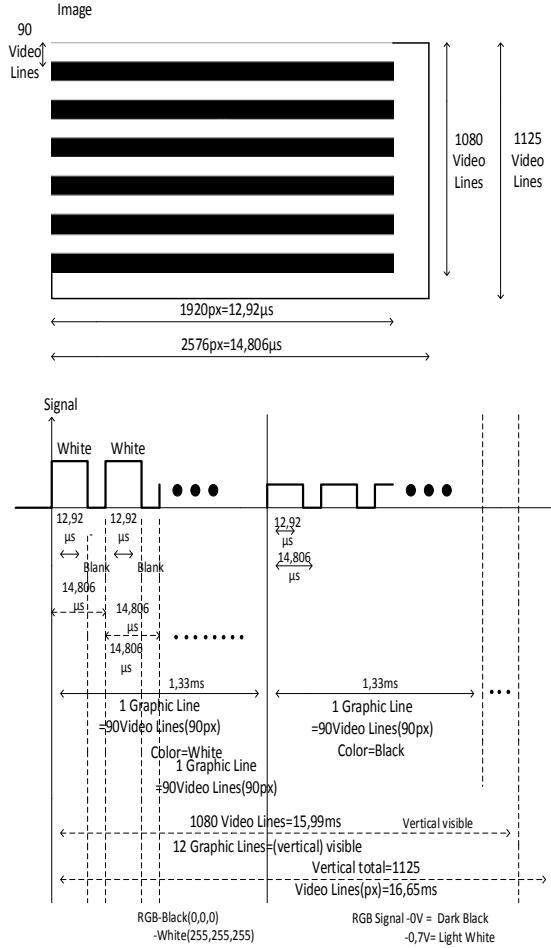
Fig. 2. The structure of the 6 white stripes and 6 black stripes - video resolution of 1920 x 1080 at 60 (Hz) refresh rate
