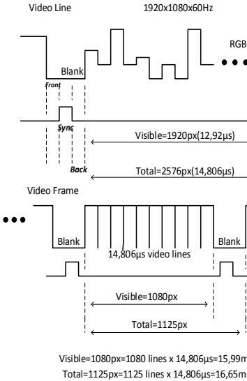
Fig. 1. The structure of an analogical video signal for the 1920 x 1080 resolution at 60 (Hz) refresh rate
