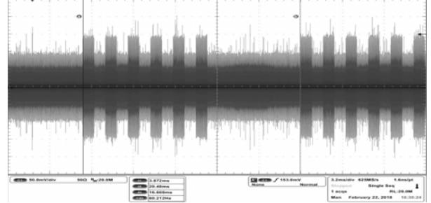
Fig. 6. Video signal - 6 horizontal lines, using MDS-21 clamp and a commercial power cable
