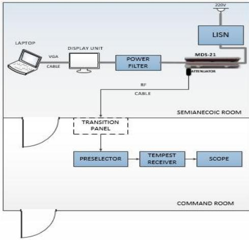
Fig. 3. Test configuration setup – MDS21 measurements
