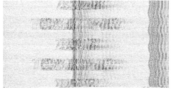
Fig. 11. Video signal recovery – no EUT, VGA cable in proximity of power line cable
