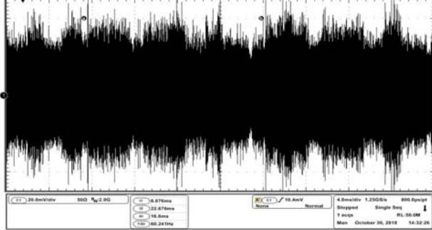
Fig. 8. Video signal - two thick horizontal bars and a thin one, using a LISN and a shielded power supply
