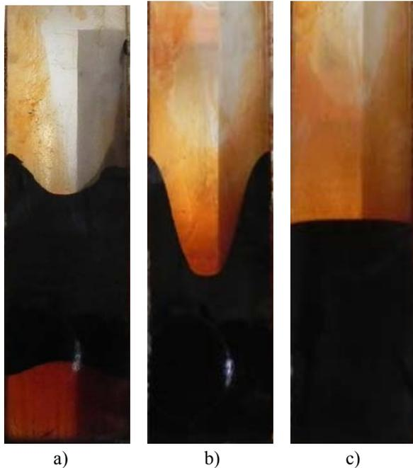
Fig. 12. The magnetic liquid rise, for: a. the ferrofluid sample having the base placed in the nonuniform field; b. the ferrofluid sample placed in the uniform field; c. the ferrofluid sample having the free surface placed in the nonuniform field.
