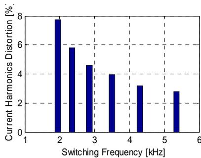
Fig. 16. Current Total Harmonics Distortion versus switching frequency
