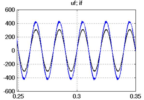
Fig. 13. The grid voltage (black) and current (blue)
