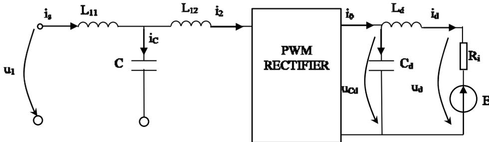
Fig. 6. Single line diagram of the battery charging system.
