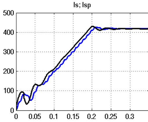
Fig. 11. The peak grid current: prescribed as controller output (black) and real (blue).
