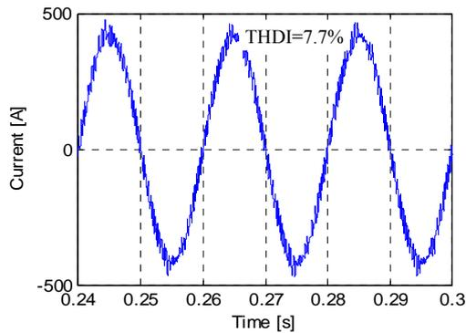
Fig. 15. The grid current corresponding to 1.95 kHz switching frequency
