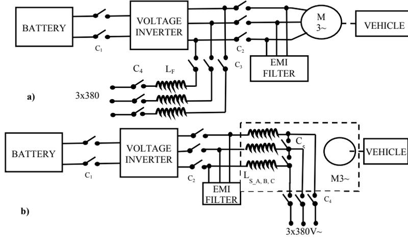
Fig. 1. Variants of use the traction inverter of an autonomous vehicle to charge the battery: a) with additional energy storage ( $L_F$ ); b) using stator coils as an energy accumulator.
