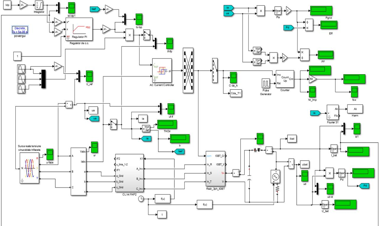
Fig. 8. The Simulink model of the control and power system.
