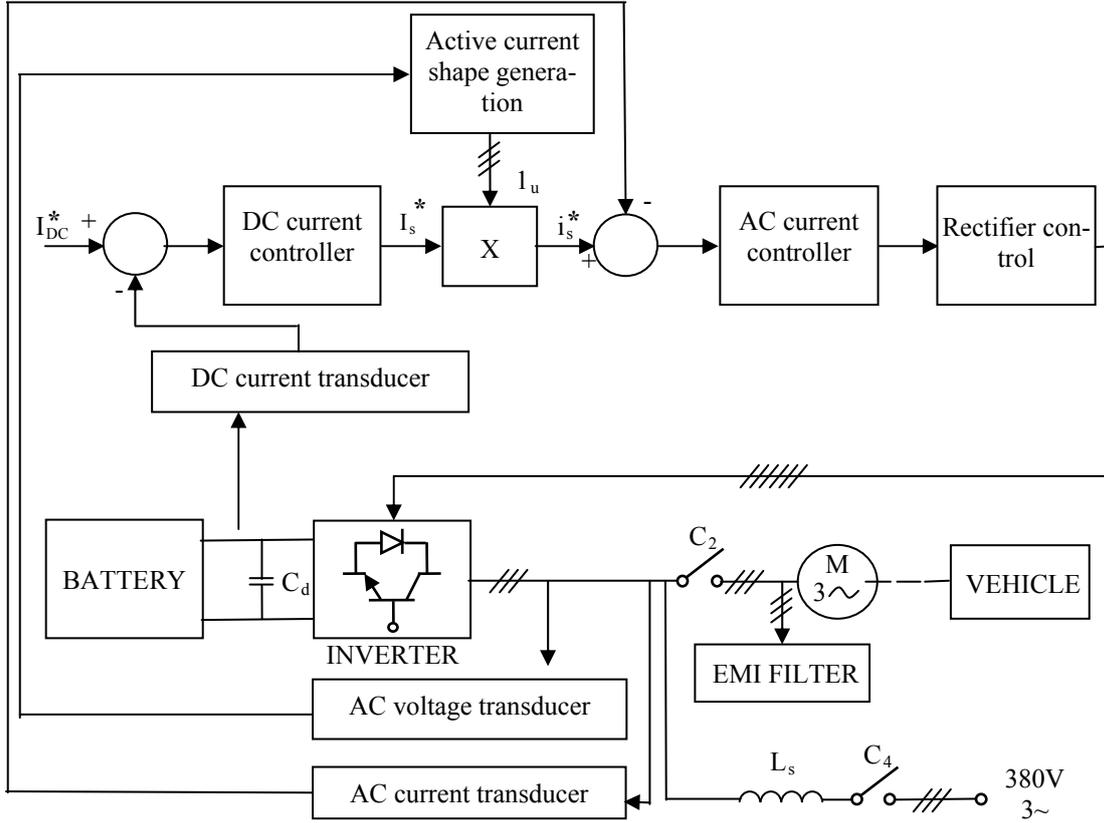
Fig. 5. Direct grid current control with two current loops.
