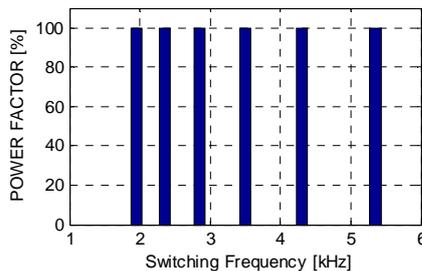
Fig. 16. Total Power Factor versus switching frequency
