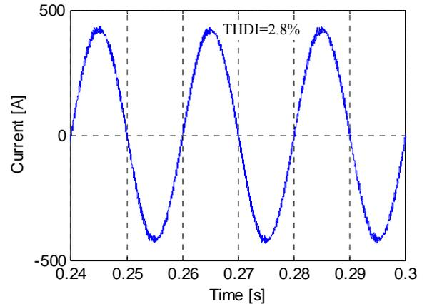
Fig. 14. The grid current corresponding to 5.35 kHz switching frequency
