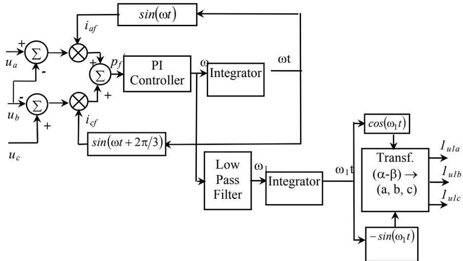
Fig. 4. Structure of the PLL circuit for the template of the grid current generating.
