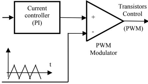
Fig. 3. Structure of the PI Current controller with PWM Modulator.
