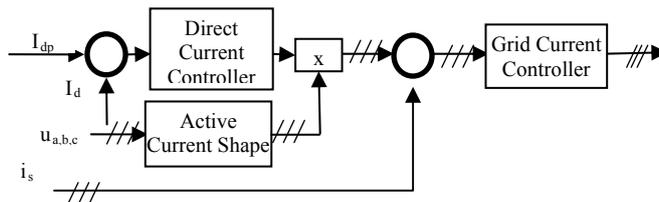
Fig. 2. Block diagram of the direct current control.
