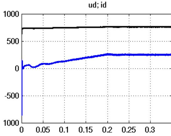
Fig. 10. The battery voltage (black) and current (blue).
