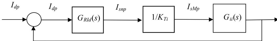
Fig. 7. Operational diagram of the battery charging current loop with unitary reaction.
