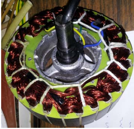
Fig.2. View with the magnetic core and the winding in a brushless direct current motor.
