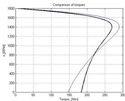
Fig. 12. Speed- torque curves for double (black line) and single cage rotor
