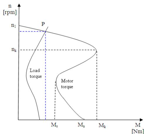
Fig. 1. Characteristic torque-speed curve of the squirrel cage induction
