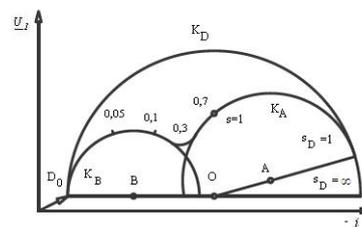
Fig.6. Circle diagram for a double cage rotor
