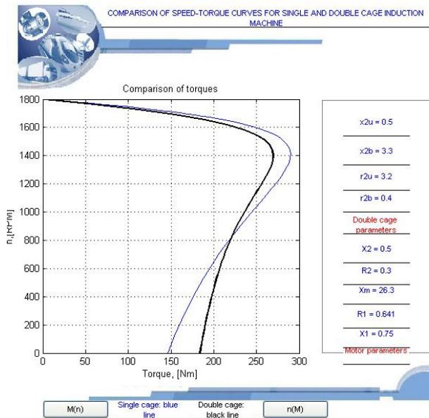
Fig. 15. Speed- torque curves called by interface
