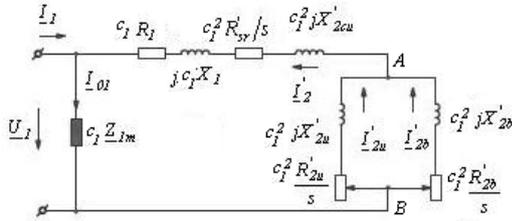
Fig.7. Equivalent schema with the magnetization circuit taken out to the terminals for a double cage rotor
