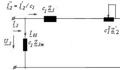
Fig.9. Equivalent schema with the magnetization circuit taken out to the terminals for the single cage rotor
