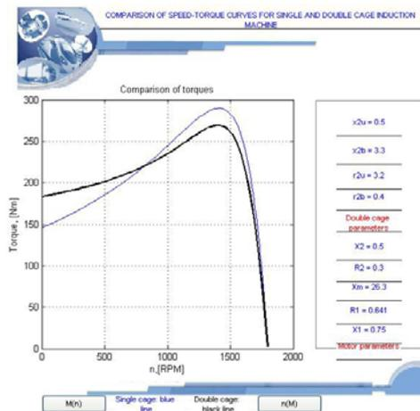
Fig. 14. Torque-speed curves called by interface
