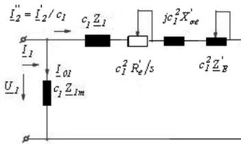
Fig.8. Equivalent schema with the magnetization circuit taken out to the terminals for a double cage rotor
