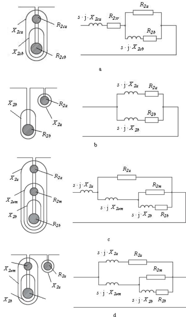
Fig.3. Slots and equivalent schemas of multiples cages rotors: a-b double cage, c-d-triple cage
