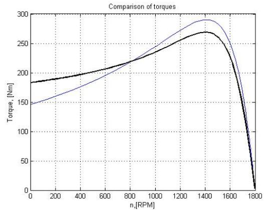
Fig. 13. Torque-speed curves for double (black line) and single cage rotor
