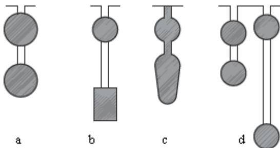
Fig. 2. Slots of multiples cages shape: a-c double cage, d-triple cage
