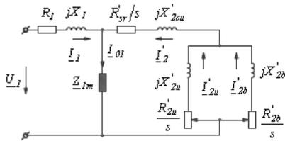
Fig.4. Equivalent schema in T for a double cage rotor with separate short-circuit rings
