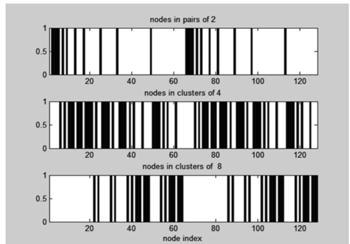
Fig. 5. Distribution of odd harmonic orders considering the clustering patterns.
