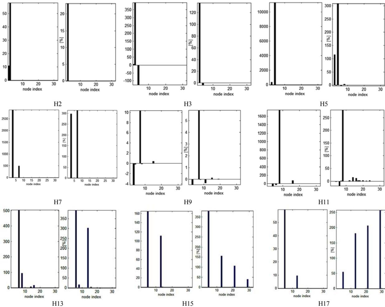
Fig. 13. Graphs G1 (left) and G2 (right), labeled Hx, associated to the energies of terminal nodes when varying the harmonic order Hx, with x in the set {2,3,4,5,7,9,11,13,15,17}
