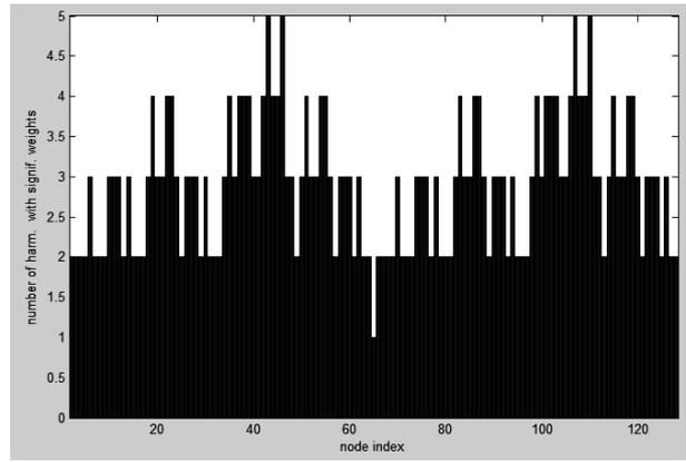
Fig. 4. Number of odd harmonic orders with more than 1% from their energy affecting the node.
