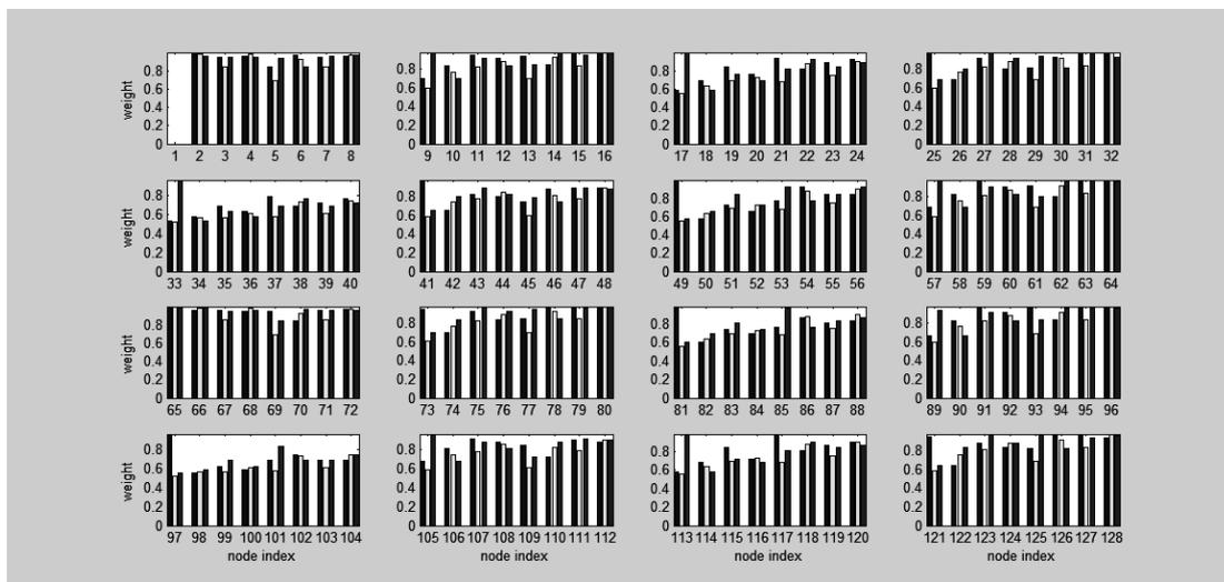
Fig. 10. Highest harmonic weights associated to node clustering patterns based on the most significant harmonic orders.
