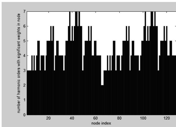
Fig. 6. Number of even harmonic orders with significant weights in nodes.
