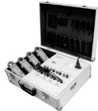
Fig. 2. Portable data acquisition system used to acquire data.
