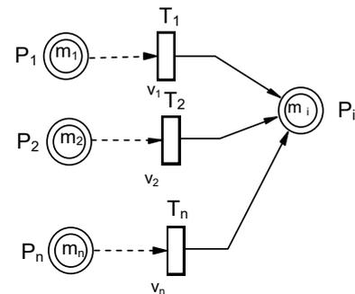
Fig.3 Continuous place with „ $n$ ” input transitions.
