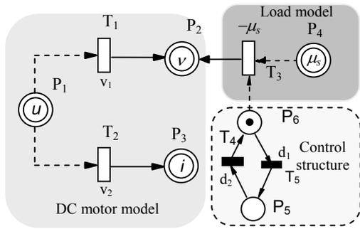
Fig.9 The Hybrid Petri net model of the electric DC drive working in an intermittent operating regime, with a constant load.
