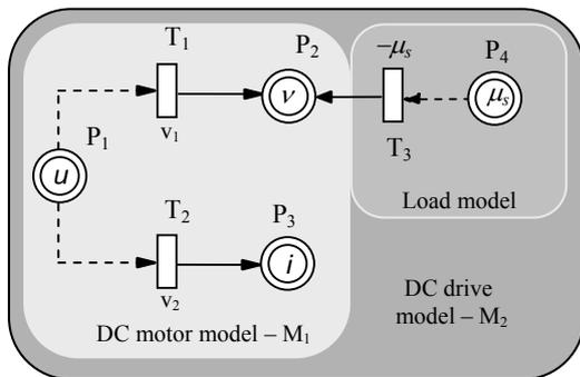
Fig.7 The MPN model of an DC electric drive for  $\mu_s = 1$ .
