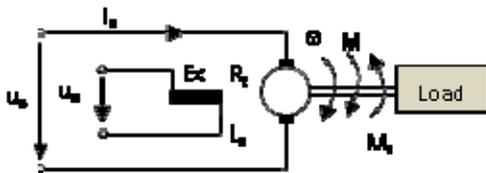
Fig.4 An DC motor drive structure
