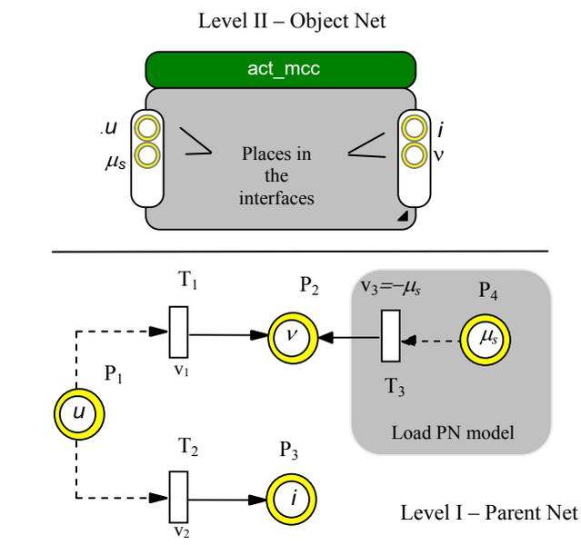
Fig.12 The Object Net built from the initial parent MPN model.
