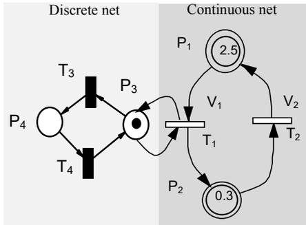
Fig.1 A Hybrid Petri net structure.
