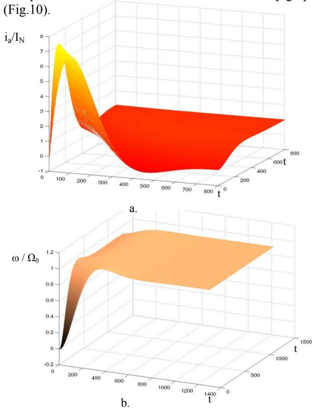
Fig.10 The reachability graphs of the hybrid system: a) rotor current; b) angular velocity.
