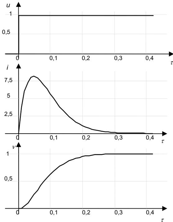
Fig.6 The transient regime during the starting process ( $\mu_s = 0$ ) reached by simulating the MPN model of an DC electrical drive, using the VisualObjectNet++ tool.
