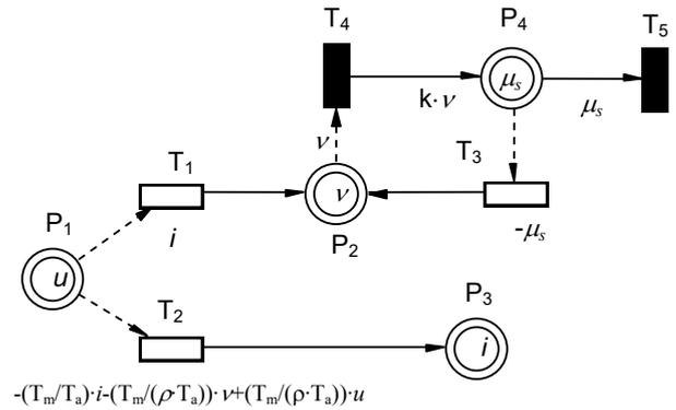
Fig.11 DC electric drive MPN model for  $\mu_s = k \cdot v$ .
