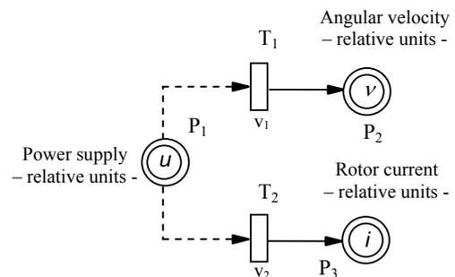
Fig.5 MPN model of an DC electrical drive for  $\mu_s = 0$
