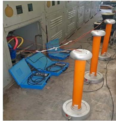
Fig. 6. Current and voltage measurement acquisition system.
