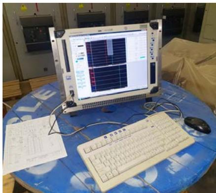
Fig. 6. TRAS Mobile acquisition system.
