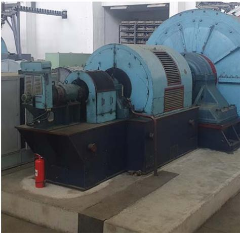
Fig. 5. Asynchronous motor with wound rotor, type ATM 2500 -2
